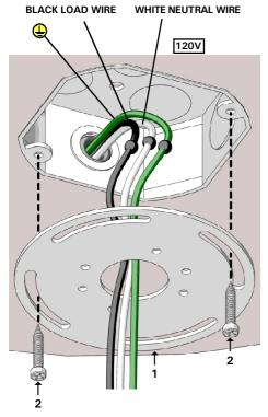
Make the cables coming from the fixture go through the hole in plate (1). Make the electrical connections between the white cable coming from the fixture and the white cable of the j-box, and between the black cable coming from the fixture to the black cable of the j-box. Also connect the green cable coming from the fixture to the green cable of the j-box. Fasten plate (1) to the j-box by means of the two screws (2).
