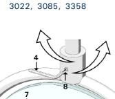
To adjust the position of diffuser (7), loosen dowel (8) by means of the Allen screw (4) supplied.
