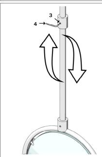
For models 3085 and 3358, before installing the fixture, adjust the telescopic stem at the desired height by loosening dowel (3) by means of the Allen wrench (4) supplied and cut the exceeding cable.
