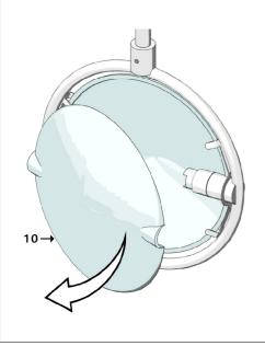
Replace the bulb by inserting it into the lamp holder and avoiding touching it with bare hands. Put glass (10) again and fix it by means of springs (9).
