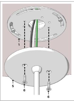
Fix the lamp body (5) to plate (1) by means of the two screws (6).
