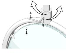
To replace the bulb, rotate diffuser (7) to a horizontal position, unhook springs (9) and take off glass (10).
